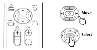
To navigate on the on-screen menus, use the "arrow" buttons  $(\diamondsuit, \diamondsuit, \diamondsuit, \diamondsuit)$  to move the cursor. Pressing these arrows will cause the cursor to move in the corresponding direction. Pressing center button ( ) will allow you to select an option.
